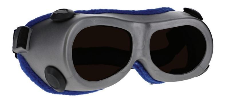
The IPLB laser safety glasses have a polycarbonate brown lens filter that provides laser protection. These laser glasses have visible light transmission of 11%. In addition, the IPLB laser safety glasses have ANSI Z87.1 and ANSI Z136.1 safety standards. These laser safety goggles 55 is a durable and lightweight fitover goggles frame. Made of high-quality plastic, the 55 laser safety goggles feature a strap. These Phillips Safety laser safety goggles are available in silver.
