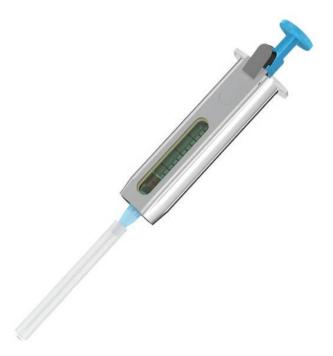
Phillips Safety's Nuclear Medicine Syringe Shield for 5ml syringes is built to provide reliable radiation protection in nuclear medicine environments. This precision-engineered shield features a compact design crafted from a dense tungsten alloy, offering dependable safety without sacrificing usability.
