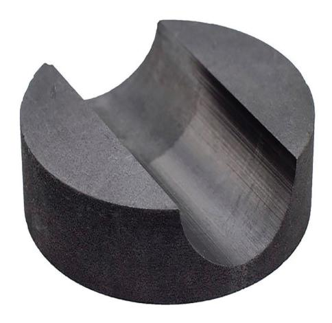
The Small Radial Head Parallel Masher is a replacement head designed specifically for the Parallel Masher. It is made of high-quality graphite and has an internal diameter measurement of 1.75", with a 5/8" wide head indent. Please note that the Small Radial Head Parallel Masher is sold individually so that replacement of chipped or broken sides is easy and affordable. If you need one complete set, remember to get two heads.
