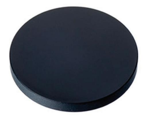
Ultraviolet Transmitting, Visible Absorbing Filters transmit the ultraviolet region but absorb the visible region. These filters are chiefly used for single extraction of ultraviolet rays. They are often utilized for selectively transmitting the 253.7 nm and 365 nm wavelengths, which are the representative line spectra of mercury lamps. Application: Medical, Inspection Device, Lighting
