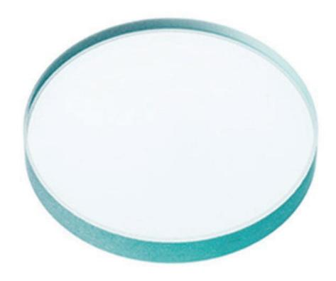
Heat Absorbing Filters feature high transmittance in the visible region and good absorption of heat rays (infrared rays). They efficiently absorb thermal radiation emitted from light sources and are highly effective when employed for slide projectors and illumination equipment. To prevent a Filter Glass from being broken by rapid heating or cooling, this filter can be also provided as a thermal toughening tempered glass. Application: Medical
