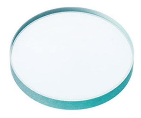
Heat Absorbing Filters feature high transmittance in the visible region and good absorption of heat rays (infrared rays). They efficiently absorb thermal radiation emitted from light sources and are highly effective when employed for slide projectors and illumination equipment. To prevent a Filter Glass from being broken by rapid heating or cooling, this filter can be also provided as a thermal toughening tempered glass. Application: Medical
