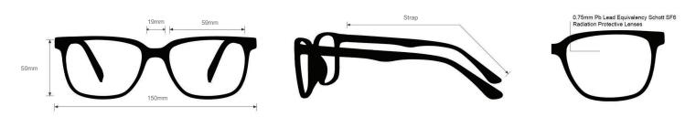
The radiation glasses 55 feature high quality, distortion-free SF-6 Schott glass radiation-reducing lenses with 0.75mm Pb lead equivalency protection. The 55 lead glasses have clear CE Certified Lens and weight 158 g. These radiation goggles 55 are non-prescription. Made of high-quality plastic, it is a durable and lightweight fitover goggles frame. The 55 radiation goggles feature strap. These Phillips Safety radiation goggles are available in silver.
