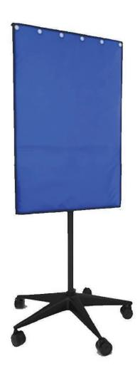
The Mobile Lead Porta-Shields provides a convenient and effective way to protect personnel or patients agains radiation. It sits on a heavy duty, five-caster base, which offers a sturdy, 24-inch diameter, ensuring smooth and stable transportation around the room. An adjustable telescoping hole allows the shield height to be set by the user and can be as low as 36 inches or as high as 56 inches. The shield's 0.5 mm lead equivalency meets industry standards for medical x-ray protection.
