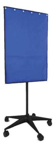
The Mobile Lead Porta-Shields provides a convenient and effective way to protect personnel or patients agains radiation. It sits on a heavy duty, five-caster base, which offers a sturdy, 24-inch diameter, ensuring smooth and stable transportation around the room. An adjustable telescoping hole allows the shield height to be set by the user and can be as low as 36 inches or as high as 56 inches. The shield's 0.5 mm lead equivalency meets industry standards for medical x-ray protection.
