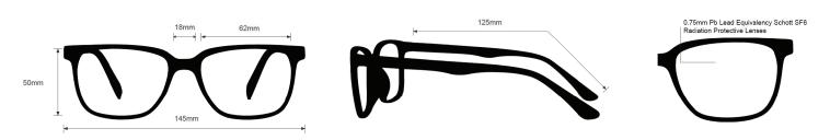
The Radiation Glasses ESC302N feature high quality, distortion-free SF-6 Schott glass radiation-reducing lenses with 0.75mm Pb lead equivalency protection. These lead glasses also provide 0.50mm Pb lead equivalency lateral protection. The ESC302N lead glasses have clear CE Certified Lens and weight 114g. These extra large radiation glasses are non-prescription, and are available in black. Made of high-quality plastic, it is a durable and lightweight fit over frame.
