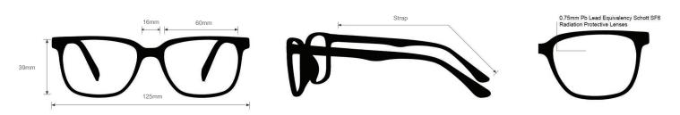
The radiation glasses RK2 feature high quality, distortion-free SF-6 Schott glass radiation-reducing lenses with 0.75mm Pb lead equivalency protection. The RK2 lead glasses have clear CE Certified Lens and weight 85 g. These radiation goggles RK2 are prescription available. Made of high-quality plastic, it is a durable and lightweight goggles frame. The RK2 radiation goggles feature foam eyecup and strap. These Phillips Safety prescription radiation goggles are available in black.
