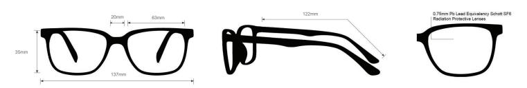
The radiation glasses 8483 feature high quality, distortion-free SF-6 Schott glass radiation-reducing lenses with 0.75mm Pb lead equivalency protection. The 8483 lead glasses have clear CE Certified Lens and weight 71g. These radiation glasses 8483 are non-prescription. Made of high-quality plastic, it is a durable and lightweight wrap around frame. The 8483 radiation glasses feature rubberized nosepad and temples bars. These Phillips Safety radiation glasses are available in black and green.
