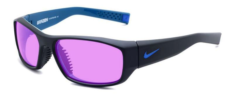
The lampworking glasses Phillips 202 have a glass violet lampworking lens that provides excellent color recognition for soft glass. These flameworking glasses offer excellent UV blocker, good IR protection, excellent sodium flare blocker, and excellent clarity. Recommended for those who work with lampwork or hot glass in small pieces.
