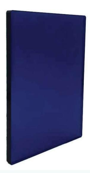
The Cobalt Blue Neotherm Glass Welding Window is a sheet made of glass that absorbs UV Radiance and harmful Infrared Emissions in the 780 to 2000nm range. It can be used for furnace and glory hole observation and is available in Cobalt Blue Neotherm shades 4, 5, 6 and 8. These Phillips Safety Neotherm lenses are certified to EN 166 and EN 171 standards.
