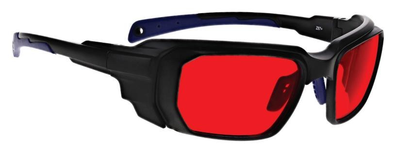
The AA laser safety glasses have a polycarbonate red lens filter that provides laser protection. These laser glasses have visible light transmission of 26%. In addition, the AA laser safety glasses have ANSI Z87.1 and ANSI Z136.1 safety standards. These laser safety glasses 16001 is a durable and lightweight wrap around frame. Made of high-quality plastic, the 16001 laser safety glasses feature adjustable nosepads. These Phillips Safety laser safety glasses are available in black/blue.
