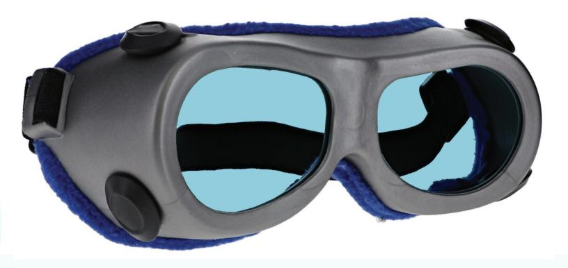
The BGKG laser safety glasses have a glass light blue lens filter that provides laser protection. These laser glasses have visible light transmission of 50%. In addition, the BGKG laser safety glasses have ANSI Z87.1 and ANSI Z136.1 safety standards. These laser safety goggles 55 is a durable and lightweight fitover goggles frame. Made of high-quality plastic, the 55 laser safety goggles feature strap. These Phillips Safety laser safety goggles are available in silver.
