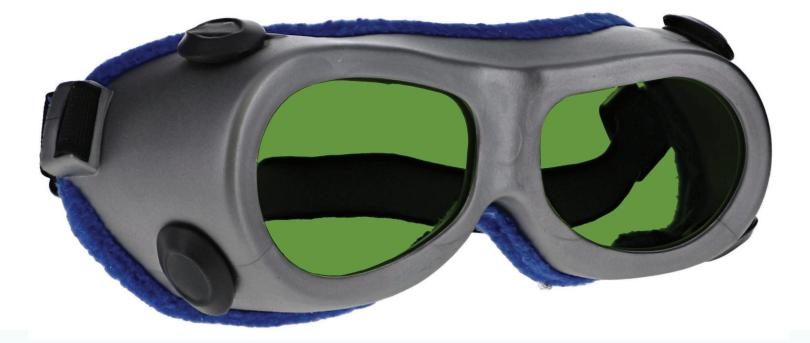
The Y93 laser safety glasses have a polycarbonate green lens filter that provides laser protection. These laser glasses have visible light transmission of 41%. In addition, the Y93 laser safety glasses have ANSI Z87.1 and ANSI Z136.1 safety standards and CE certified lens. These laser safety goggles 55 is a durable and lightweight fitover goggles frame. Made of high-quality plastic, the 55 laser safety goggles feature strap. These Phillips Safety laser safety goggles are available in silver.
