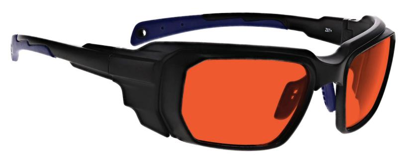
The AKP laser safety glasses have a polycarbonate orange lens filter that provides laser protection. These laser glasses have visible light transmission of 46.4%. In addition, the AKP laser safety glasses have ANSI Z87.1 and ANSI Z136.1 safety standards. These laser safety glasses 16001 is a durable and lightweight wrap around frame. Made of high-quality plastic, the 16001 laser safety glasses feature adjustable nosepads. These Phillips Safety laser safety glasses are available in black/blue.
