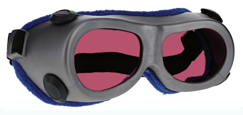
The AD laser safety glasses have a polycarbonate pink lens filter that provides laser protection. These laser glasses have visible light transmission of 32.6%. In addition, the AD laser safety glasses have ANSI Z87.1 and ANSI Z136.1 safety standards. These laser safety goggles 55 is a durable and lightweight fitover goggles frame. Made of high-quality plastic, the 55 laser safety goggles feature strap. These Phillips Safety laser safety goggles are available in silver.
