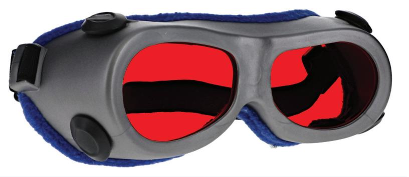
The AA laser safety glasses have a polycarbonate red lens filter that provides laser protection. These laser glasses have visible light transmission of 26%. In addition, the AA laser safety glasses have ANSI Z87.1 and ANSI Z136.1 safety standards. These laser safety goggles 55 is a durable and lightweight fitover goggles frame. Made of high-quality plastic, the 55 laser safety goggles feature strap. These Phillips Safety laser safety goggles are available in silver.
