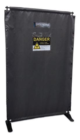
The LaserEdge is a laser safety barrier that protects 120W/cm<sup>2</sup> for 100 seconds, with a wavelength of 1070nm and 1mm diameter spot (1/e). With a lightweight design, this laser safety barrier has the exclusive LaserEdge technology, with a single panel and integrated light-blocking strip.
