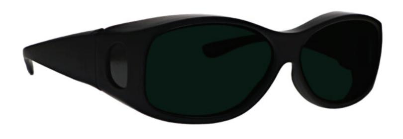
The lampworking glasses Boroview 3.0 have a polycarbonate green glassworking lens that provides good color recognition for borosilicate glass and furnace work. These flameworking glasses offer excellent UV blocker, excellent IR protection, excellent sodium flare blocker, and good clarity. Recommended for those who work with lampwork or hot glass in small pieces.
