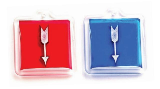
The Square X-Ray Markers with Arrow are high-quality radiographic film identification markers to mark X-Ray films. With a square shape, they feature lead arrows and are color coded, one marker being blue and the other red. The arrows are completely embedded in crystal clear epoxy.
