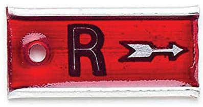
The L&R X-Ray Markers with Arrow are high-quality radiographic film identification markers to mark X-Ray films. With a rectangular horizontal shape, they feature color coded lead letters to indicate left and right, with L being blue and R red. In addition, they have lead arrows on both sides. Both the letters and the arrows are completely embedded in crystal clear epoxy.
