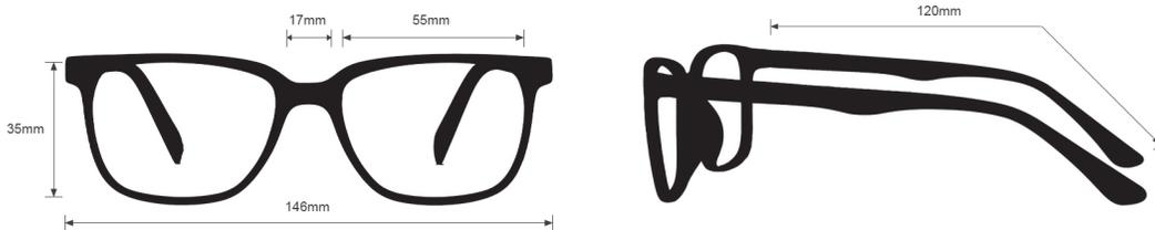
The Safety Glasses Q300 are a rectangular, wrap around frame made of high-quality plastic. The Q300 model is lightweight, highly durable, and impact resistant. Plus, it features rubberized nosepads, rubberized temple bars, and side shields. These Safety Glasses are available in black. They also meet rigorous industry standards, with ANSI Z87+ and EN 166, offering high impact certification for optimal protection.
