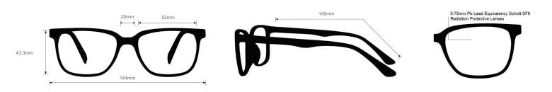
The radiation glasses Nike Radeon 2 feature high quality, distortion-free SF-6 Schott glass radiation-reducing lenses with 0.75mm Pb lead equivalency protection. The radiation safety glasses Nike Radeon 2 have clear CE Certified Lens and weight 57.3g. These radiation glasses Nike Radeon 2 are prescription available. Made of high-quality plastic, it is a durable and lightweight rectangular frame. Plus, these Nike lead glasses feature rubberized temple bars and are available five colors.
