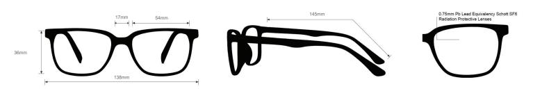
The radiation glasses Nike 7057 feature high quality, distortion-free SF-6 Schott glass radiation-reducing lenses with 0.75mm Pb lead equivalency protection. The radiation safety glasses Nike 7057 have clear CE Certified Lens and weight 42.3g. These radiation glasses Nike 7057 are prescription available. Made of high-quality plastic, it is a durable and lightweight rectangular frame. These Nike lead glasses feature rubberized temple bars and are available in four colors.
