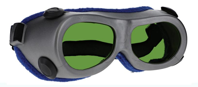
The Y93 laser safety glasses have a polycarbonate green lens filter that provides laser protection. These laser glasses have visible light transmission of 41%. In addition, the Y93 laser safety glasses have ANSI Z87.1 and ANSI Z136.1 safety standards and CE certified lens. These laser safety goggles 55 is a durable and lightweight fitover goggles frame. Made of high-quality plastic, the 55 laser safety goggles feature strap. These Phillips Safety laser safety goggles are available in silver.
