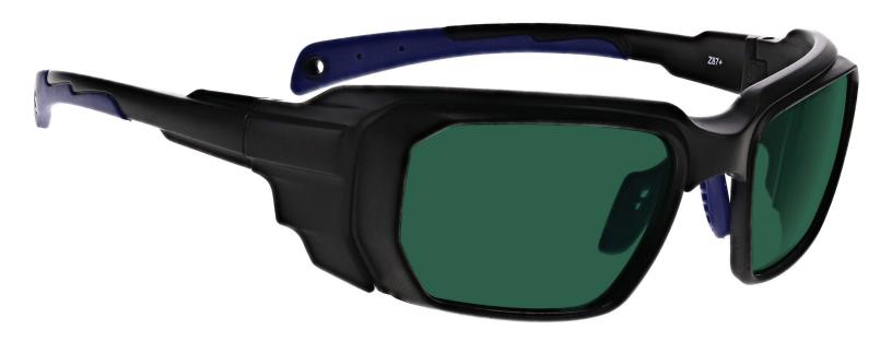
The DIO laser safety glasses have a polycarbonate green lens filter that provides laser protection. These laser glasses have visible light transmission of 2.8%. In addition, the DIO laser safety glasses have ANSI Z87+ plus ANSI Z136.1 safety standards. These laser safety glasses 16001 is a durable and lightweight wrap around frame. Made of high-quality plastic, the 16001 laser safety glasses feature adjustable nosepads. These Phillips Safety laser safety glasses are available in black/blue.
