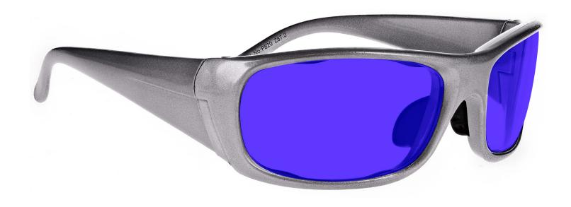
The lampworking glasses Sodium Flare Poly have a polycarbonate purple glassworking lens that provides good color recognition for soft glass. These flameworking glasses offer excellent UV blocker, good IR protection, excellent sodium flare blocker, and good clarity. Recommended for those who work with lampwork or hot glass in small pieces.
