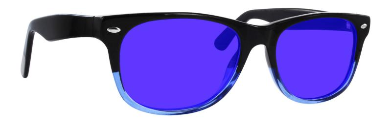
The lampworking glasses Sodium Flare Poly have a polycarbonate purple glassworking lens that provides good color recognition for soft glass. These flameworking glasses offer excellent UV blocker, good IR protection, excellent sodium flare blocker, and good clarity. Recommended for those who work with lampwork or hot glass in small pieces.
