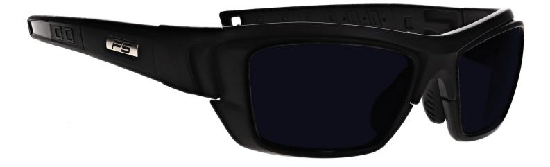
The lampworking glasses BoroTruView 5.0 have a polycarbonate dark navy glassworking lens that provides excellent color recognition for borosilicate glass. These flameworking glasses offer excellent UV blocker, excellent IR protection, excellent sodium flare blocker, and excellent clarity. Recommended for those who work with lampwork or hot glass in large pieces.
