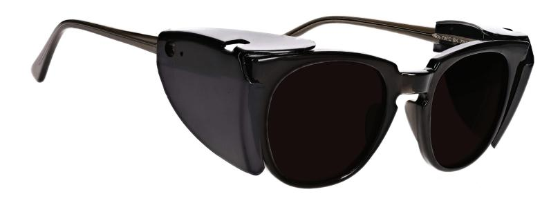
The lampworking glasses Boroview 5.0 have a polycarbonate brown glassworking lens that provides good color recognition for borosilicate glass. These flameworking glasses offer excellent UV blocker, excellent IR protection, excellent sodium flare blocker, and good clarity. Recommended for those who work with lampwork or hot glass in large pieces.
