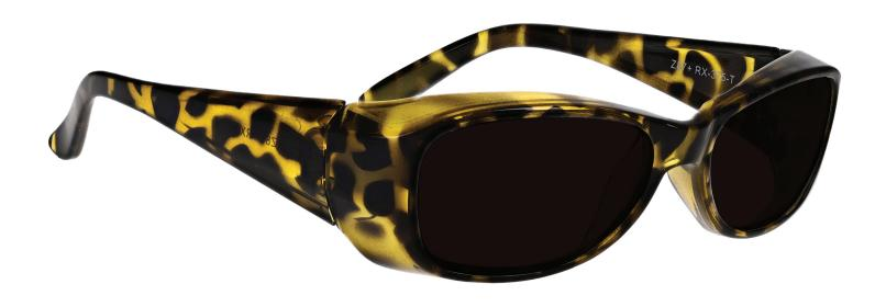
The lampworking glasses Boroview 5.0 have a polycarbonate brown glassworking lens that provides good color recognition for borosilicate glass. These flameworking glasses offer excellent UV blocker, excellent IR protection, excellent sodium flare blocker, and good clarity. Recommended for those who work with lampwork or hot glass in large pieces.
