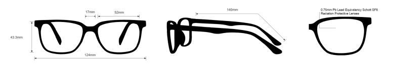
The radiation glasses Nike 7164 feature high quality, distortion-free SF-6 Schott glass radiation-reducing lenses with 0.75mm Pb lead equivalency protection. The radiation safety glasses Nike 7164 have clear CE Certified Lens and weight 75g. These radiation glasses Nike 7164 are prescription available. Made of high-quality plastic, it is a durable and lightweight cat eye, oval frame. These Nike lead glasses feature a saddle bridge and are available in four different colors.
