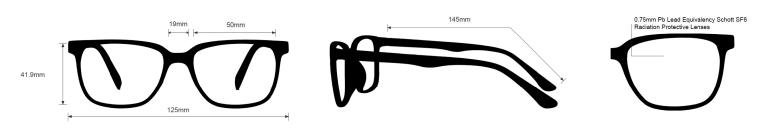
The radiation glasses Nike 7162 feature high quality, distortion-free SF-6 Schott glass radiation-reducing lenses with 0.75mm Pb lead equivalency protection. The radiation safety glasses Nike 7162 have clear CE Certified Lens and weight 65g. These radiation glasses Nike 7162 are prescription available. Made of high-quality plastic, it is a durable and lightweight oval frame. Plus, these Nike lead glasses feature rubberized temple bars and are available in four different colors.
