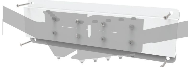
Note: The concrete anchor must be able to support 150lbs
