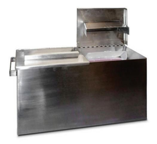
The Shielded Sharps Container provides a simple, safe and convenient solution for the disposal of used syringes that may be contaminated with high-energy radionuclides. It features convenient lifting handles and has a key-lockable, hinged top. With 0.5 and 1.0 inch lead shielding, it accommodates any size sharps container. As with all of our products, Phillips Safety can design and manufacture a custom shielded sharps container to meet your exact specifications.
