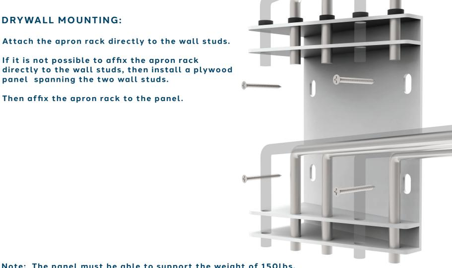
Note: The panel must be able to support the weight of 150lbs.
